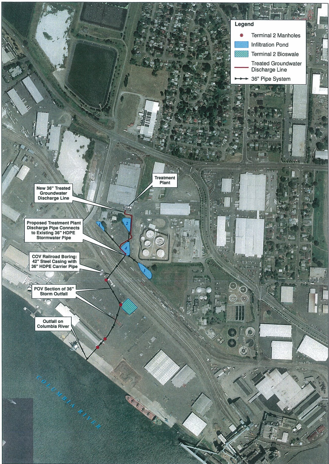
Figure 1 Existing 36-inch Stormwater Outfall
