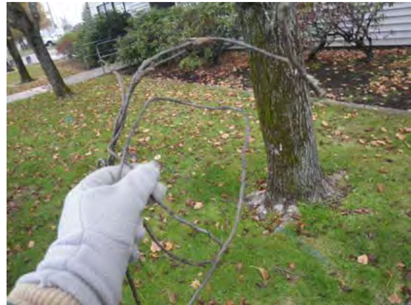
Photo 8. Twisted wire found in bore hole B2 at 7.6 m (25 ft) below the surface.
